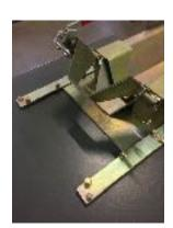
6. The side extensions can be mounted by inserting the square tube channel into the center table.
