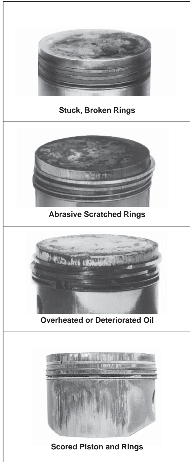
Figure 10-12. Common Types of Piston Damage.
