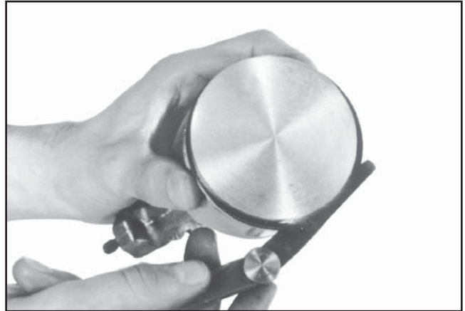
Figure 10-14. Measuring Piston Ring Side Clearance.
